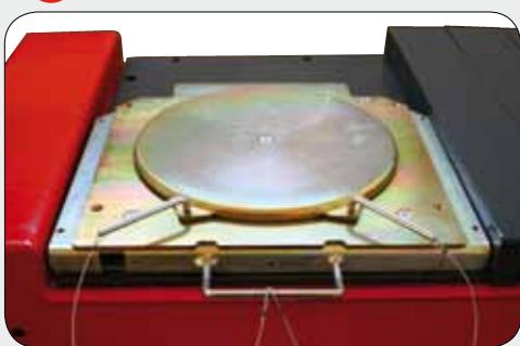
**(EN)** The recesses for the turn plates and slip plates are adjustable to ensure **perfect planarity of the runways**.
