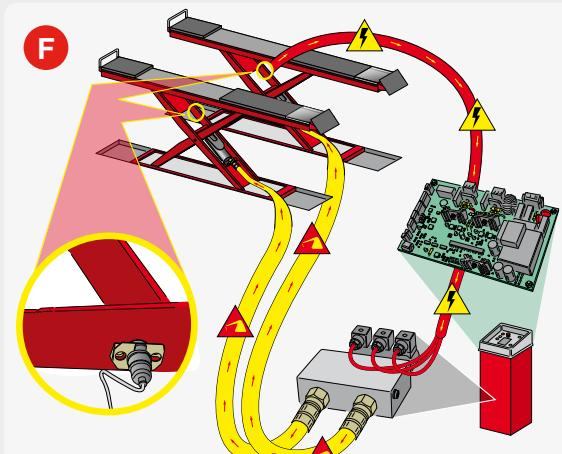
**(EN)** Electronically controlled hydraulic levelling system.
