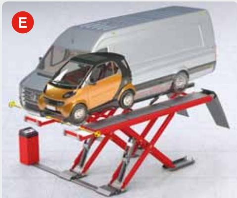
**(EN)** The vehicle's front axle is positioned in a lift's fixed point (where there are the turntables), **independently from the vehicle wheel base** and without any further regulation
